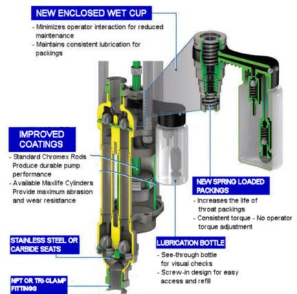
The new lowers can be used with pneumatic, hydraulic, and electric platforms. Many models have common components making cylinders and pistons easy to change between pump sizes.
