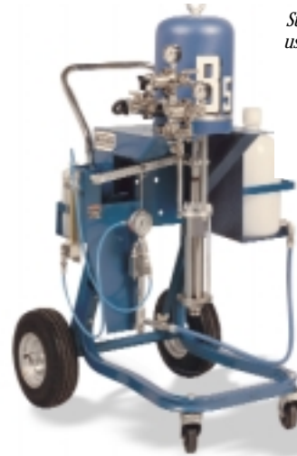
A Catalyst Flow Alarm will alert an operator to any change in catalyst or resin flow at virtually any flow rate including flow stoppage, pump failure, restrictions, air bubbles, failed seals, and surging.
